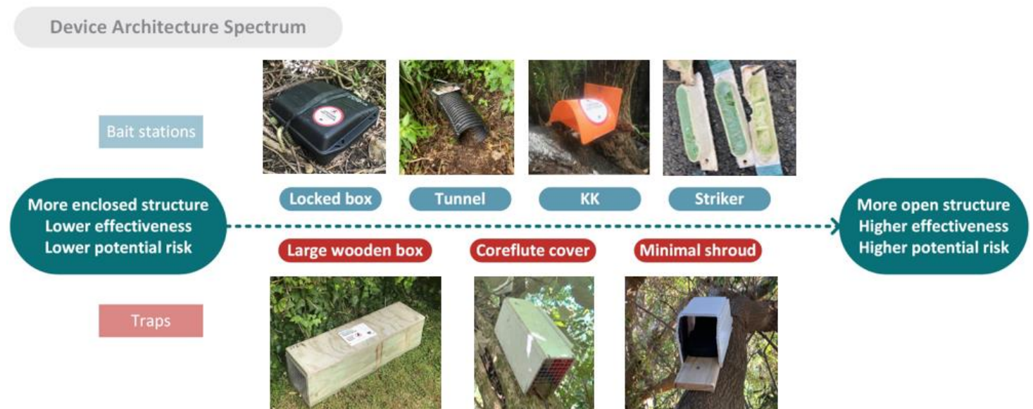
Figure 3: The spectrum of device architecture of bait stations and traps, in relation to structure, effectiveness and risk.
